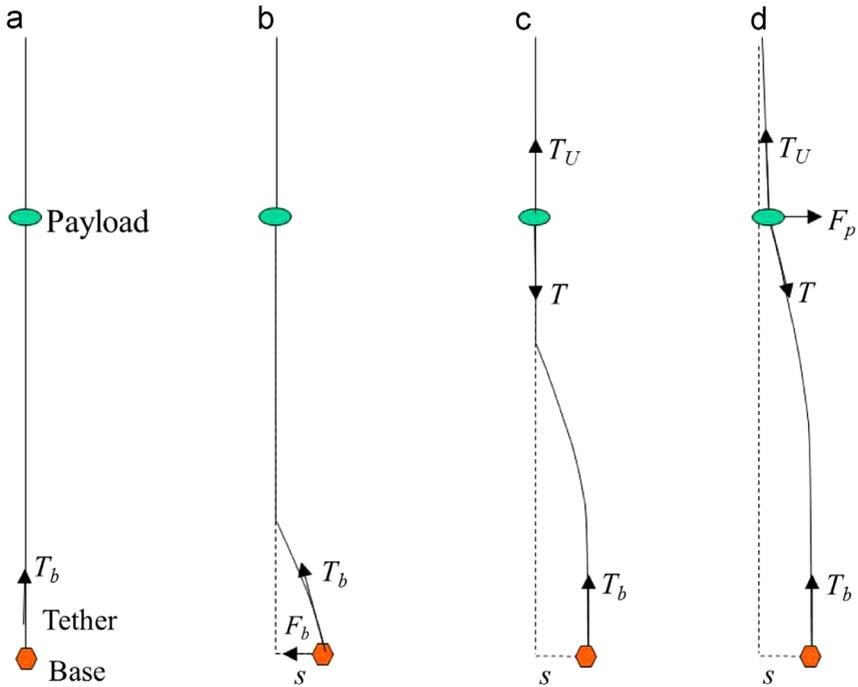
Fig. 4. Tether positions when swinging the base to avoid space debris.
